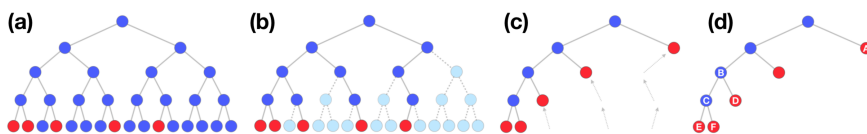
Figure 54: BIGFileFast with a binary tree: (a) Find the n = 5 most probable targets (red nodes); (b) Find their parents up to the root (dark blue nodes) and prune all the non-parent nodes (light blue nodes); (c) recursively replace the parent of a node by its child if it is the only child; (d) if the expected information gain of (A,B) is greater than that of (A,C) , prune branch C and move directly to the next branch (A,D) , skipping E and F.
